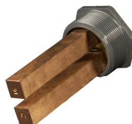
7" long 90% copper, 10% silver electrode, 3" sch 80 (*CLE-20)
