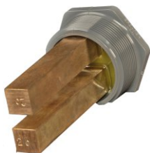
6" long 80% copper, 20% silver electrode, 3" sch 80 (*CLE-14)
